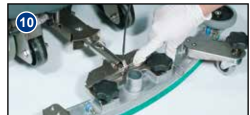
Fit the floor-tool and retain using the detent pin (Fig.9).
