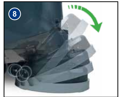
To tip the deck into the down position (Operating mode). Press in the brush deck locking pin (Fig.7) and rotate the brush deck (Fig.8).
